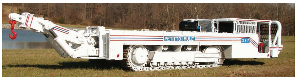
Rebuilt Diesel Petitto Mule
