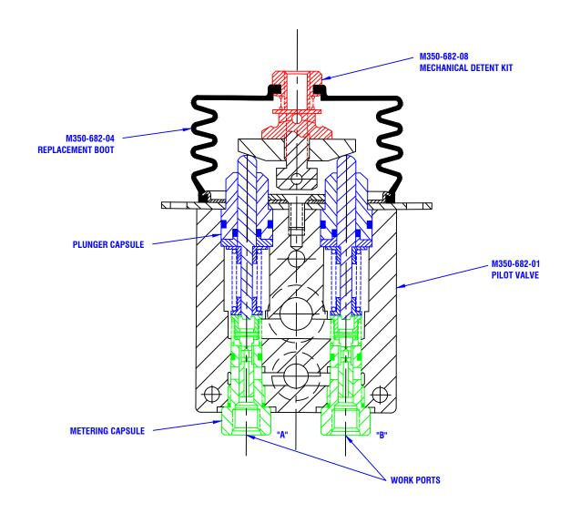
NOTE: M350-682-09 INCLUDES PILOT VALVE AND DETENT ASSEMBLY
