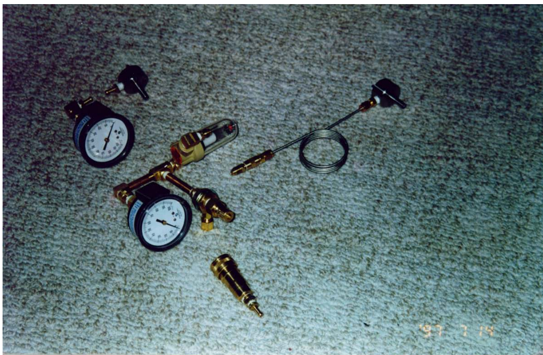
Figure 2: Components of Flameproof Port Installation
